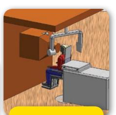
**COMING SOON! Best Proton Therapy** Cyclotron up to 150 MeV dedicated for proton therapy with two beam lines and two treatment rooms (Patent Pending)
