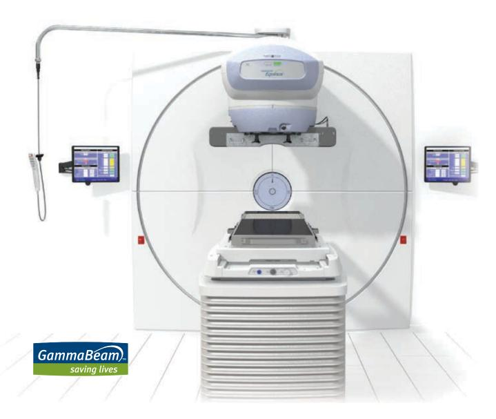
The GammaBeam 300 Equinox is an evolution of the Theratron line of treatment devices. The advanced design provides freedom in treatment planning and can interface to all of the major record and verify systems to allow for rapid treatment parameter loading, treatment set up verification, and the recording of the delivery.
